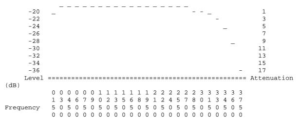
The frequency response above is for a typical good telephone line. In real life situations the high and lof frequencies can be more attenuated. The frequency curve information was taken from Dialup Line Quality in Houston web page.
