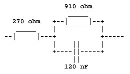
The return loss to this reference model must be greater than 15 dB.
