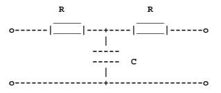
The resistor  $\mathbf{R}$  and capacitor  $\mathbf{C}$  values depend on the cable characteristics. Old Swedish telephone equipment regulations have listed the following values for simulating a typical local loop cable:
