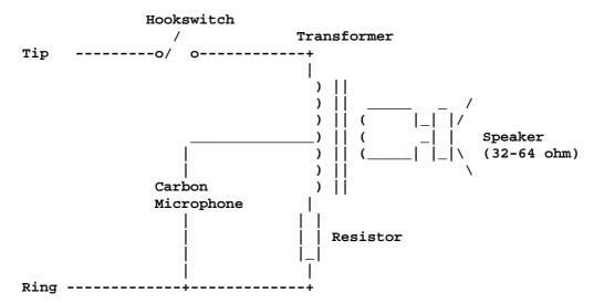
The circuit is designed so that the impedance at audio frequencies looks like about 600 ohms. The audio impedance is controlled by the transformer characteristics, carbon microphone, speaker impedance and the resistor in series with the transformer.
