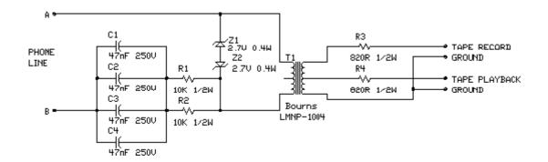
The capacitors C1 to C4 are connected in parallel to make about 200 nF capacitance. Four separate capacitors can be more easily fitted to one case than single 200 nF 250V capacitor which is quite large. I don't know the reason of why R1 and R2 are connected in parallel, because single 4.7 kohm resistor would do their job as well.
