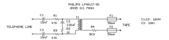
I found out the type of all other components than the transformer T1. T1 is the audio isolation transformer, which seems to have properties quite similar to typical 600:600 ohm telecom isolation transformer. The components F1 and F2 are 50mA fuses. The signal output level is suitable for microphone input because the resistors attenuate the voice signals form telephone line around 40 dB (some telephone equipment regulations in Finland needed this).
