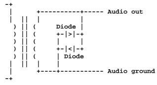
The diodes on the secondary of the transformer connected in this way will limit the signal levels to less than 0.7 Vpp.
