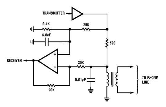
The transformer in this circuit is 600:600 ohm telephone line transformer. For best results you have to adapt the component values slightly to match the line impedance and the transformer you are using.
