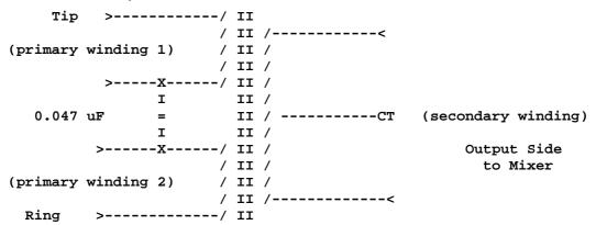
Try this circuit it works great for us in the studio. The circuit is designed to be used in paprallel with existing telephone. Just make sure you use properly rated components.
