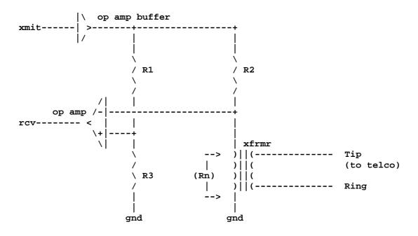
In the above diagram Rn = the telco network impedance as seen at the other side of the transformer.
