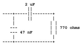
This diagram is referred to 800Hz, but impedance is rather complex, and varies from high value at low frequency and drops to ca. 150 ohm on 10kHz and 120-125 ohm above 100kHz.
