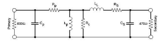
For Midcom 671-8005 tranformer the model has following parameters:
