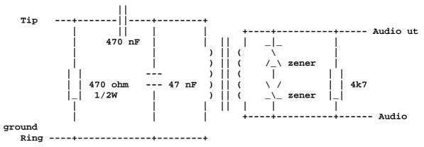
Tip and ring are first shunted with a 470 ohm 1/2 W resistor (to allow the interface to sieze the
