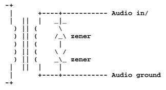
The zener diodes will limit the signals on the transformer output to around the zener diode voltage + 0.7 V range.
