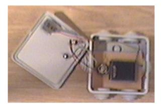
The possible uses for this circuits might be converting normal 2 wire modem for operating in 4 wire circuit (for example for connecting to radio link) or using normal telehone as microphone and speaker for computer soundcard when doing Internet telephony. If you are planning to connect the circuit to your soundcard use the following wiring:
