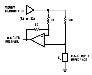
The circut below is partly redrawn optimized hybrid circuit from National Semicondictor application note "Optimum Hybrid Design" from 1985 (that application note is no longer available).
