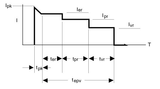
These values describe Read and rite currents but, not the maximum "power on" current. Empirically, cards have not exceeded 60mA at power up or during hot insertion and these "peaks" have not maintained these current levels for more than  $\approx 1\mu$ Sec. Q: What is the (average or peak) current draw during the 74 (or 80) initialization clock cycles?
