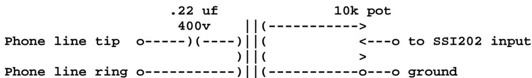
This circuit works as designed with the chip specified, because it has high impedance input. The design has one problem: If this circuit is connected to low impedance input and the output potentiometer is set to maximum level, the low impedance is reflected to primary side of the transformer, which is not good.
