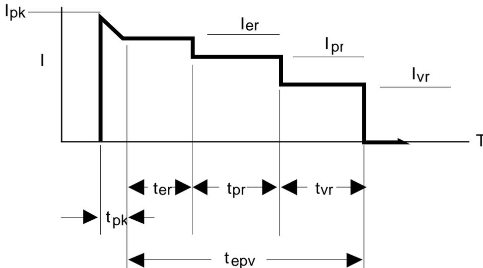
These values describe Read and rite currents but, not the maximum “power on” current. Empirically, cards have not exceeded 60mA at power up or during hot insertion and these “peaks” have not maintained these current levels for more than ≈ 1μSec.
